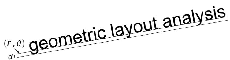
Figure 1. An illustration of Roman script text-line model proposed by Breuel.<sup>12</sup> The baseline is modeled as a straight line with parameters  $(r, \theta)$ , and the descender line is modeled as a line parallel to the baseline at a distance  $d$  below the baseline.
